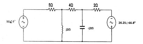
b) Find the value of load impedance 'Z' for which power transfer is (06) maximum in following circuit for w =400 rad/s & also value of max power transferred to the load.
